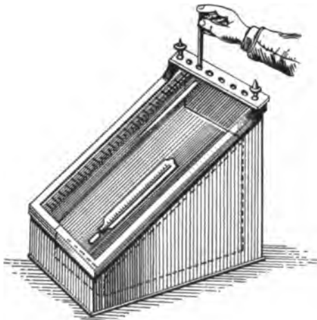
FIG 102.—Test for Gumming and Oxidation of Oil.
